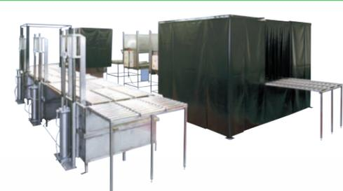
High performance integrated processing/inspection systems for fast, reliable manual penetrant testing.
